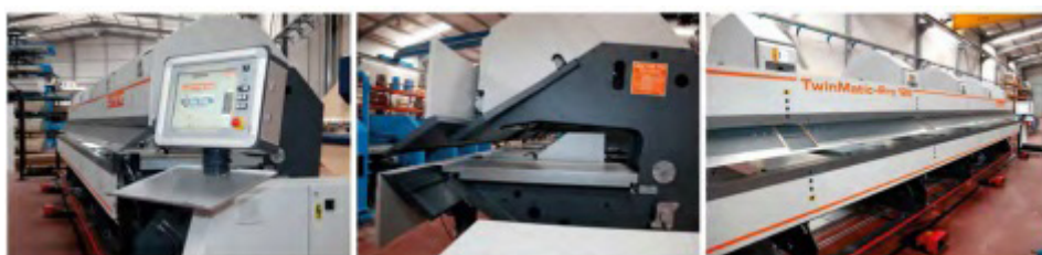
Aluminium box roll forming machines (maximum 8 metres).
