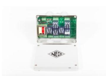
The **NECO AC Group Controller** is designed to simultaneously operate from two to eight tubular motors.
