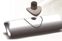
DN65~DN300, Saddle seat mounting
