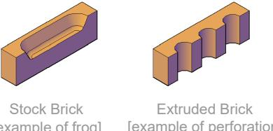
Stock Brick [example of frog]      Extruded Brick [example of perforation]
