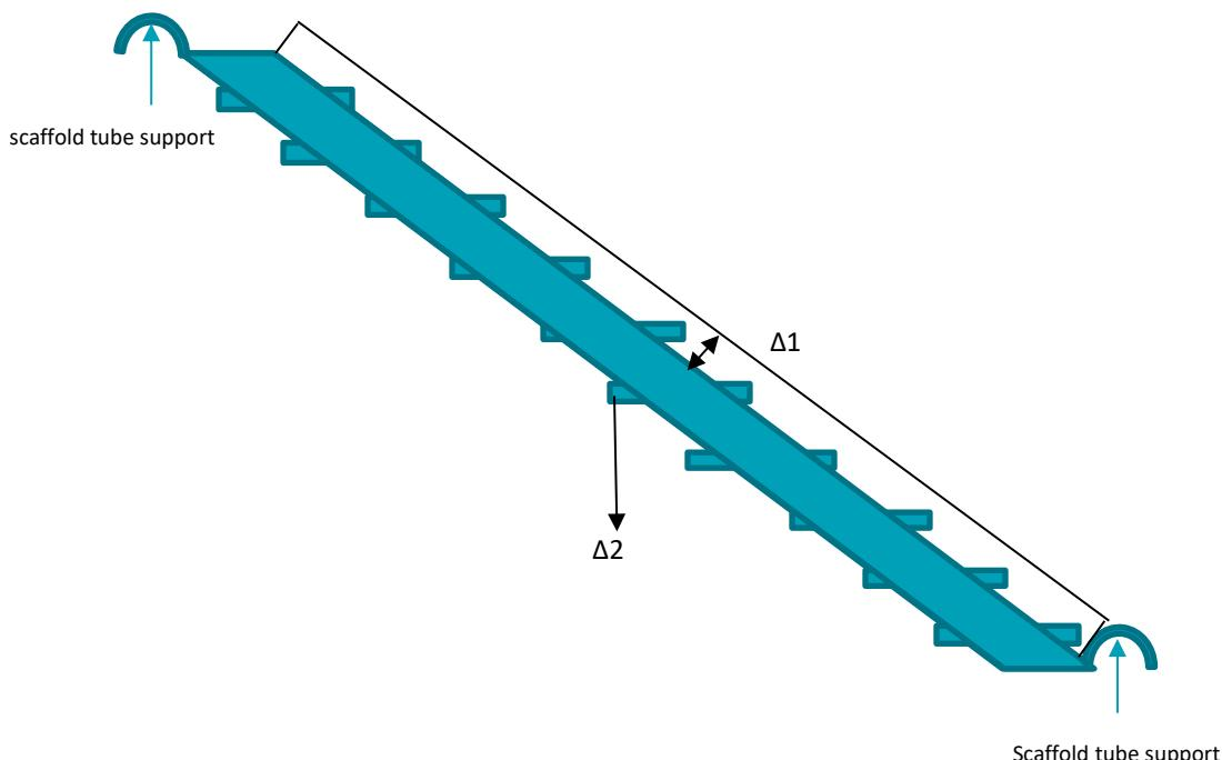
$\Delta 1$  monitoring stringer displacement,  $\Delta 2$  monitoring geometric center vertical displacement
