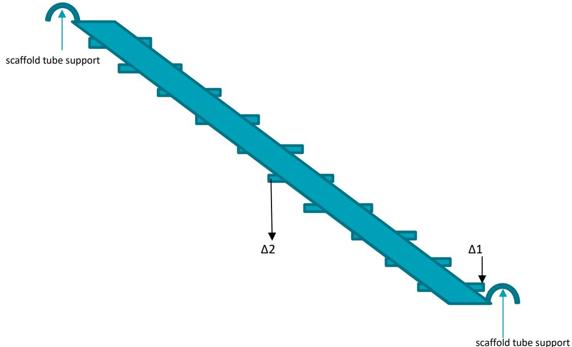
$\Delta 1$  monitoring central tread displacement,  $\Delta 2$  monitoring geometric center vertical displacement
