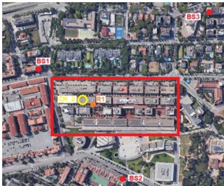
Figure 3-28: Relay control - best geographical location to place the fixed relay R1 (in orange) to address coverage hole CH_2
