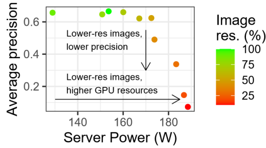
Figure 3-46: vRAN and Edge - Mean average precision vs. server's power consumption for images with different resolutions. The radio and computing resources are allocated to minimize the delay.
