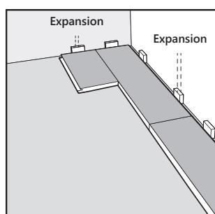
Place the spacers to ensure the correct expansion gap. For the correct expansion gaps, check the supplier installation guidelines.
