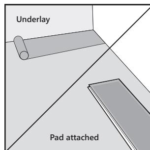
If there is no pad attached to the panels, roll out the underlayment in the same direction of the floor.
