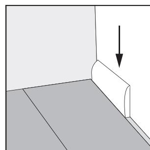
Install skirting on the walls over the expansion gaps to complete the room.
