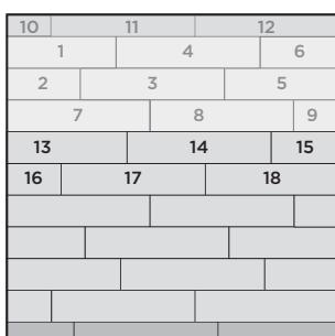
Continue installing the rest of the panels row by row in the order of the drawing.
