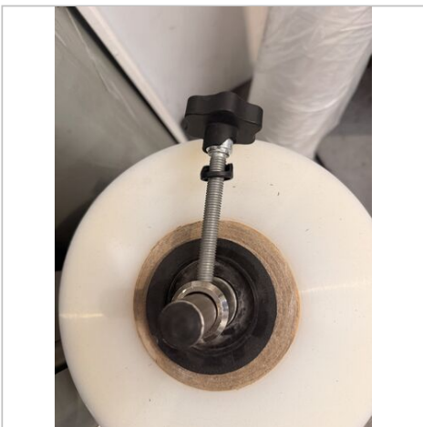
Top handle plastic broken, still functional 11 Jun 2026 11:21
